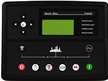
The “7420MKII” controller is an auto start mains (utility) failure module for single gen-set applications. This controller includes a backlit LCD display which continuously displays the status of the engine and generator at all times.
