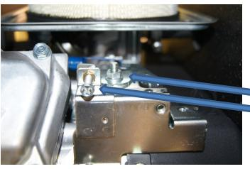
IF THE ENGINE IS NOT RUNNING AT PROPER SPEED (62HZ AT NO LOAD), THEN ANOTHER ADJUSTMENT WILL BE NEEDED. LOOSEN THE LOCK NUTS (B,C) AND TURN THE ADJUSTMENT SCREW. CW TO INCREASE SPEED OR CCW TO DECREASE SPEED. ONCE THE ENGINE IS RUNNING AT 62HZ AT NO LOAD, THEN TIGHTEN THE LOCK NUTS (C) AND THEN (B).
