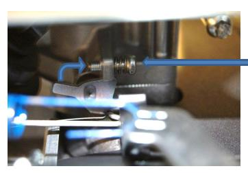
ADJUST THE THROTTLE STOP SCREW (A) SO THE ARM MAKES CONTACT. IF THIS DOES NOT LIMIT THE ARM POSITION THEN THE GOVERNOR WOULD BE ALLOWED TO OVERSHOOT.
